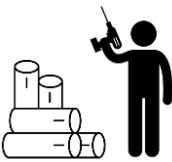
05 Drilling Lateral Holes on Both Ends of Each Tube
